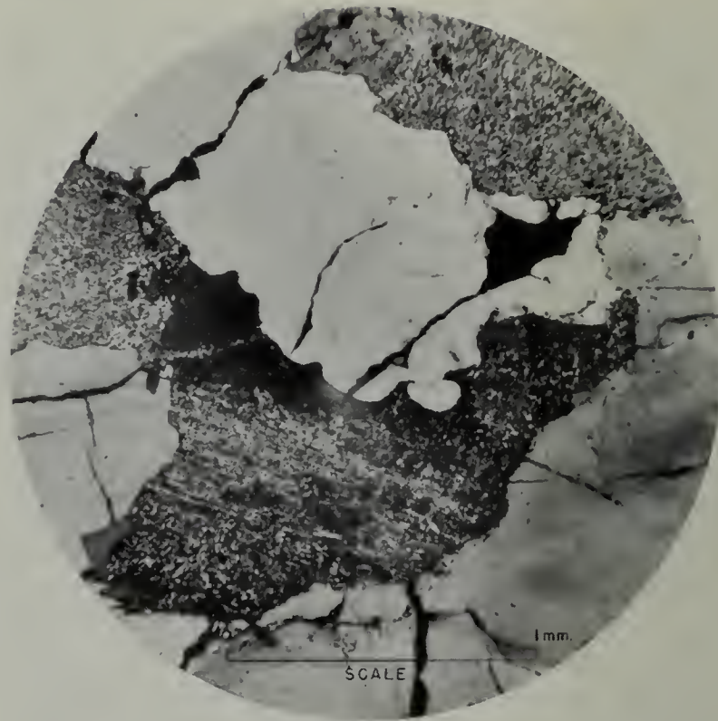
Photo 2. Biotite augen gneiss, showing quartz (white) replacing sericitized plagioclase (black), with embayed relations showing "cooky-bite" effect. Crossed nicols.
